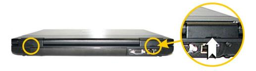
**4.** Open the lid of the mobile thin client. Using the plastic alignment tool or your finger nails, carefully pry off the switch cover starting at the corners as indicated in Figure 6.
